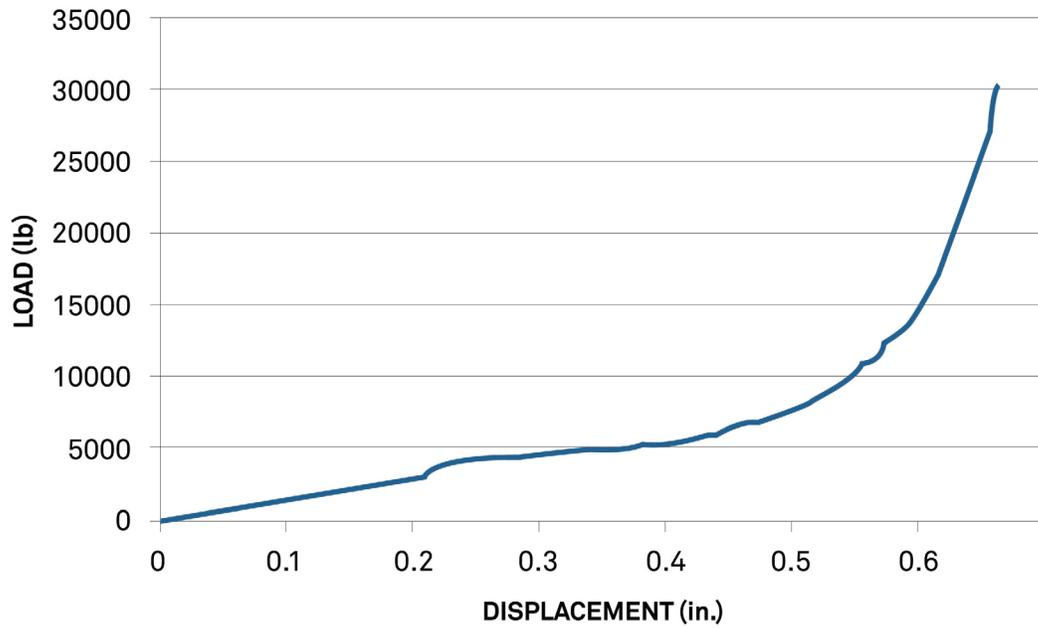
Figure 9. Load-displacement plot for sensor (horizontal orientation)
