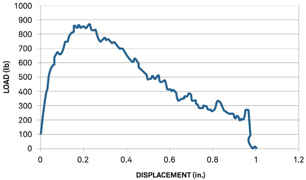
Figure 6. Load – displacement plot for Sample 2 (horizontal orientation)
