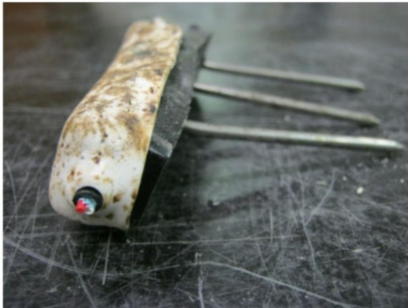
Figure 10. Sensor 2 after compression testing (horizontal orientation)
