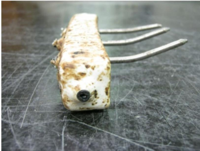
Figure 8. Sensor 1 after compression testing (vertical orientation)
