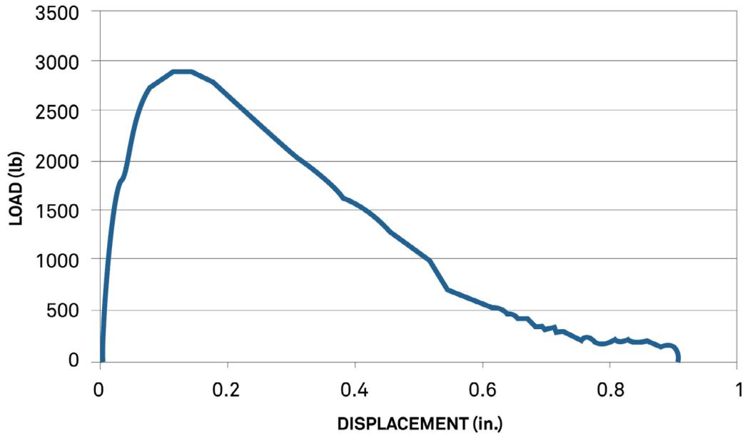
Figure 5. Load-displacement plot for Sample 1 (vertical orientation)
